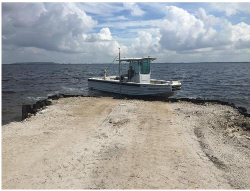
LOA: 26 ft Beam: 8 ft Power Plant: Yanmar Diesel 300 hp
